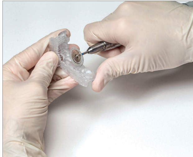
Figure 22: Remove the support structures using a cutting disc
