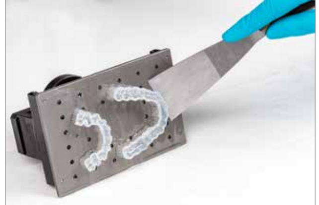
Use a spatula or cutting tool to carefully detach the printed objects from the build platform
