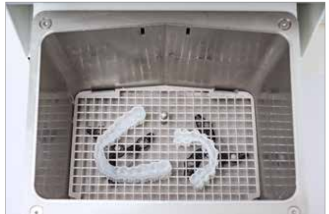
Splints in the DMG 3Dewash cleaning unit
