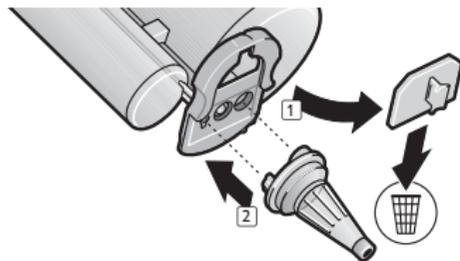
2. Remove the cap from the cartridge and discard. Attach a new mixing tip.
