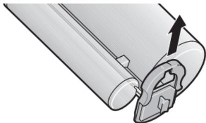
1. Slide the locking mechanism upwards in order to open the cartridge. Do not remove the locking mechanism from the cartridge.
