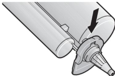
3. Secure the mixing tip by sliding the locking mechanism into the locked position.
