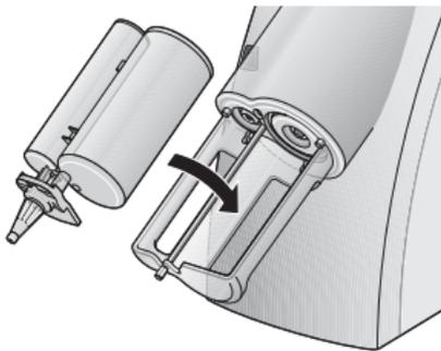
4. Insert the cartridge into the MixStar-eMotion. A brief acoustic signal confirms the correct insertion of the cartridge.
